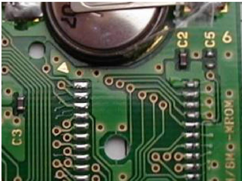
Use Rosin Flux solution and apply a small coat to each contact. Then pre-solder all connections with a very small amount of solder before connecting your wires.
