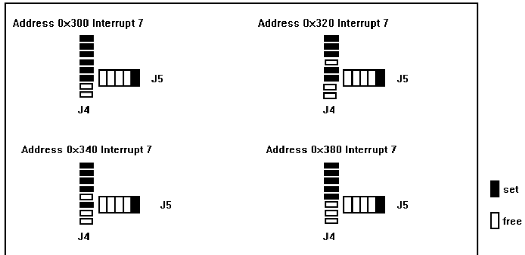
Figure 17: Jumper J4 - Address Setting
