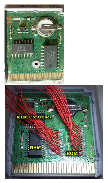
The Above images are Gamboy cartridges with onboard RAM and a Battery backup. The cartridge on the bottom is "YOSHI's BLOCKBALL" which has an **"MBC1"** memory bank controller chip.
