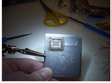
It is recommended to use 26 AWG wire or better yet, to use 30 AWG insulated wire. This will allow you to close the cartridge regardless of all the wiring work.
