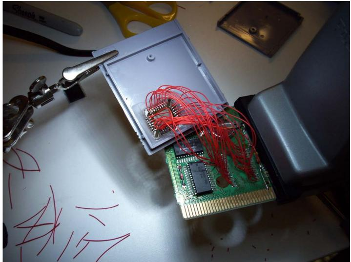
If you pre TIN your wire leads in the same manner, this will greatly improve your soldering work. Just be careful not to get to close to the adjacent contacts, a solder blob can be a pain to remove, especially if you run out of Flux and Copper wire wick.
