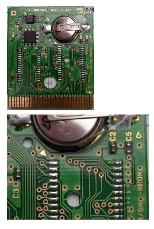
Use Rosin Flux solution and apply a small coat to each contact. Then pre-solder all connections with a very small amount of solder before connecting your wires.
