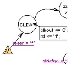
**Figure 1-21 Adding Reset Transition Condition**
