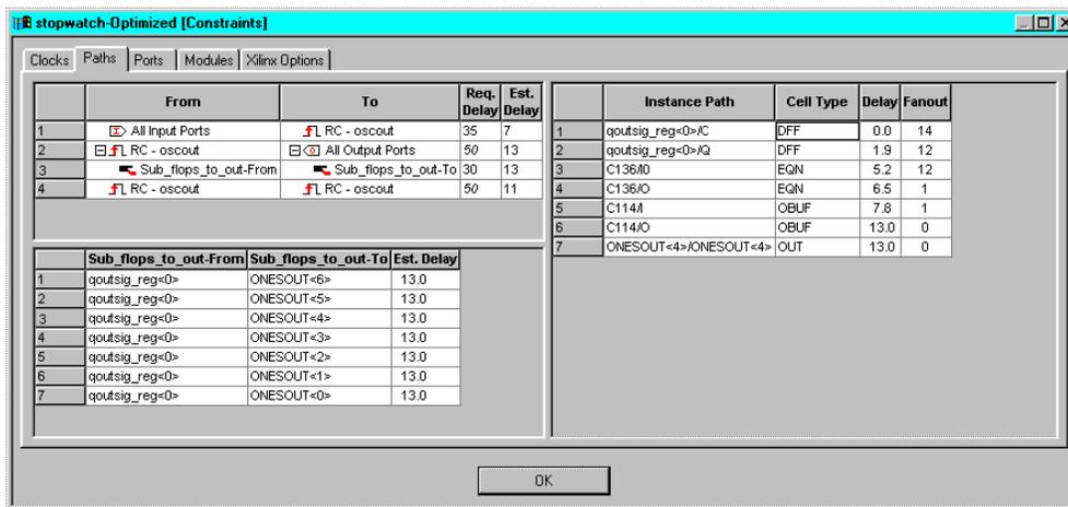
Figure 2-16 Estimated Timing Data Under Paths Tab
