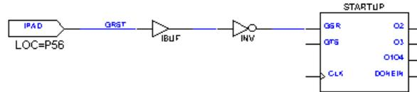
**Figure 6-4 STARTUP Symbol Connections**
