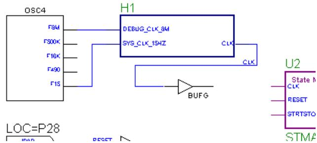
Figure 1-35 Placing the DEBUG\_CKT Macro
