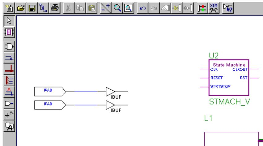
Figure 1-28 Placing RESET and STRTSTOP I/O Components
