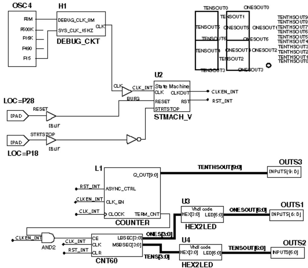
Figure 1-2 Completed Watch Schematic
