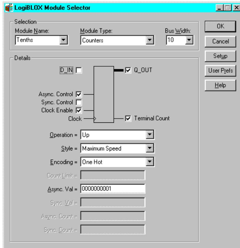
Figure 2-8 LogiBLOX Module Selector
