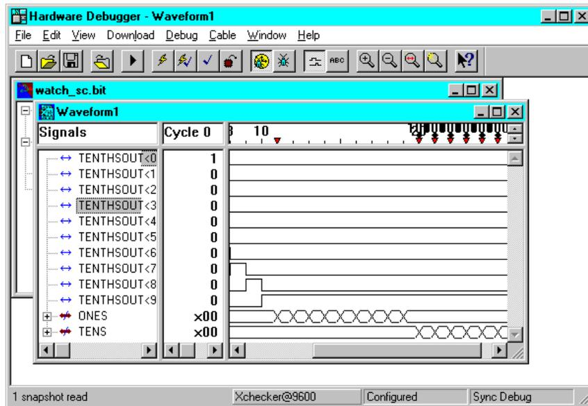
Figure 6-20 Waveform Window (Schematic Design)
