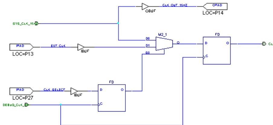
**Figure 6-5 Clock Muxing Circuitry**
