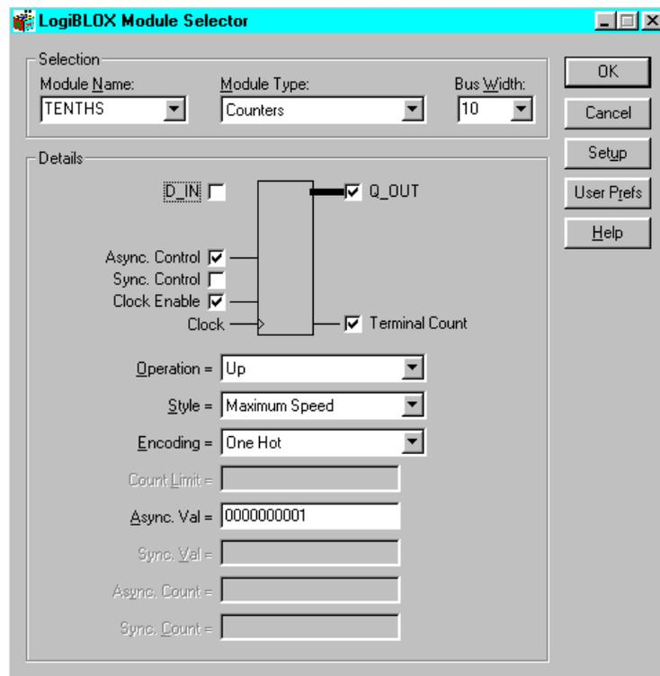
**Figure 1-14 LogiBLOX Module Selector**
