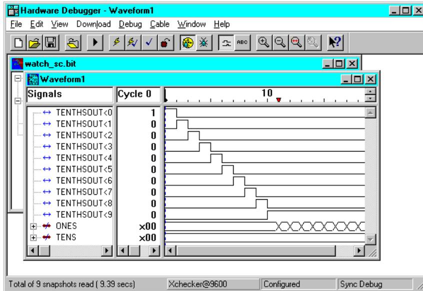
Figure 6-18 Waveform Window (Schematic Design)
