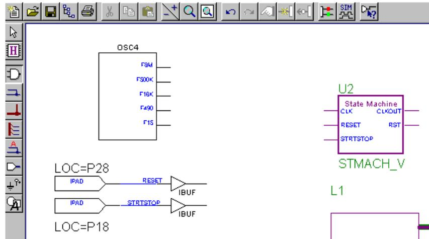
Figure 1-33 Placing the OSC4
