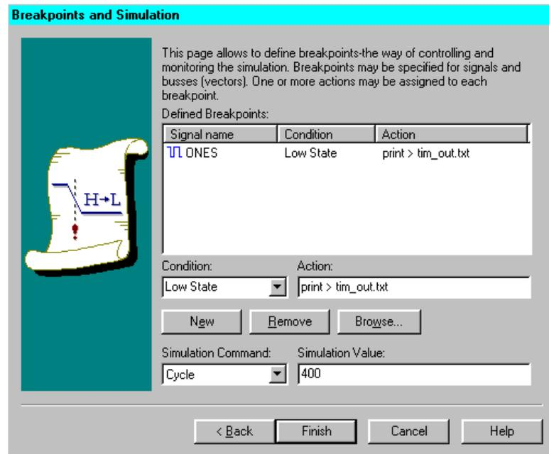
**Figure 5-7 Breakpoints and Simulation**
