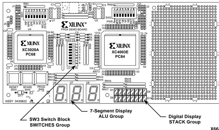
Figure 6-1 FPGA Demonstration Board Components
