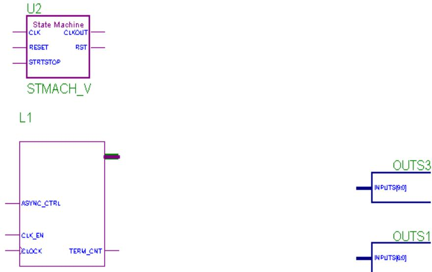
**Figure 1-22** Placing the State Machine Macro
